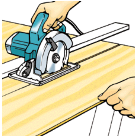
Fig. 10 Cut the 1/4-in.-thick back panel to size with a circular saw. Use a straight strip as a guide when making the cuts.
