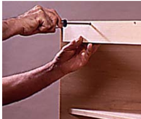
9 --Use screws and glue to join the triangular lower frames to the back frames. Bore pilot holes to avoid splitting the wood.
