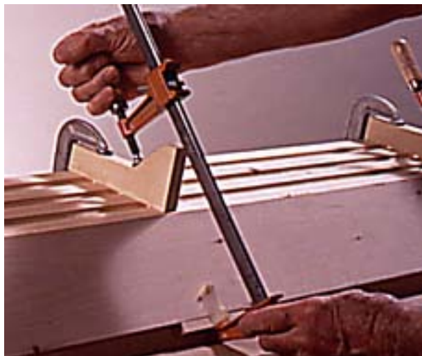
4 --Use a corebox bit and router to make the stopped flutes. A shopmade carriage supports router in correct position.
