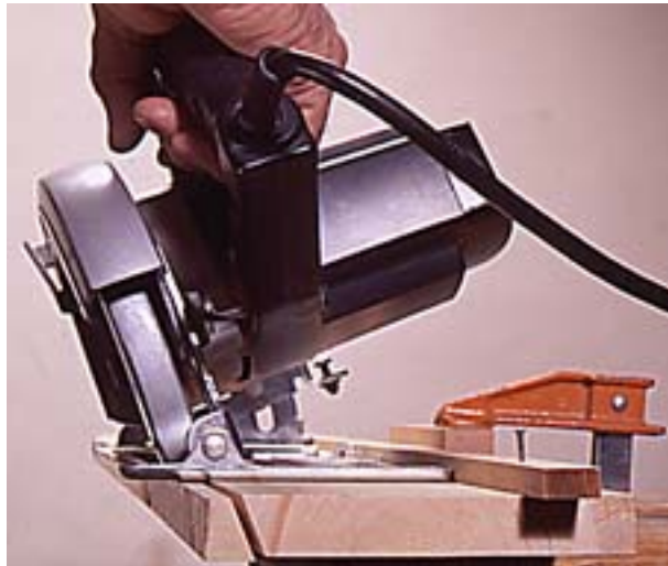
1 --Rout the half lap joints with a straight bit. Hold workpiece in a jig that has guide strips to confine the cut to the lap area.
