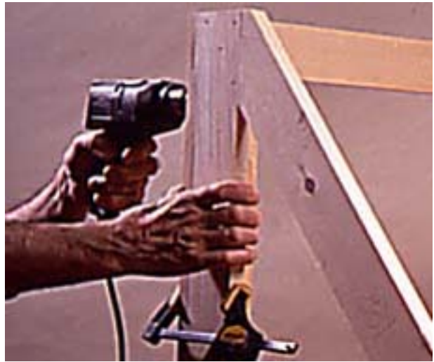
9 --Use screws and glue to join the triangular lower frames to the back frames. Bore pilot holes to avoid splitting the wood.
