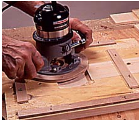
1 --Rout the half lap joints with a straight bit. Hold workpiece in a jig that has guide strips to confine the cut to the lap area.
