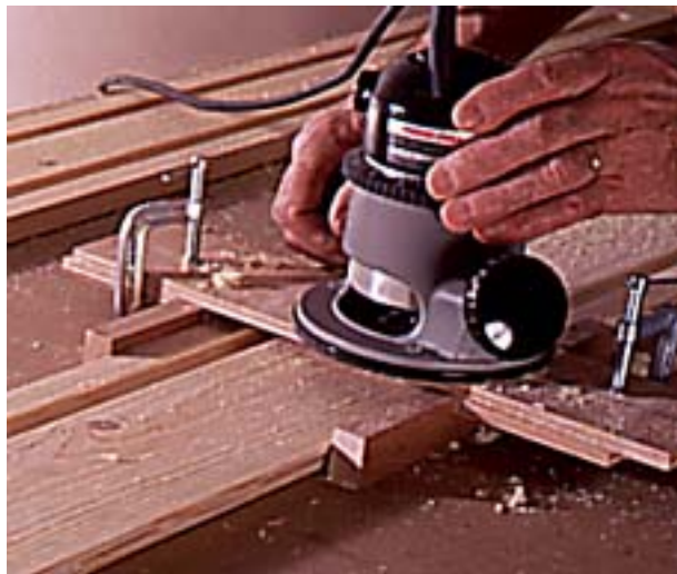
4 --Use a corebox bit and router to make the stopped flutes. A shopmade carriage supports router in correct position.
