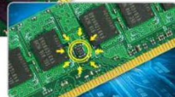
Onboard thermal sensor for better system thermal control (ECC/Registered-DIMM)
