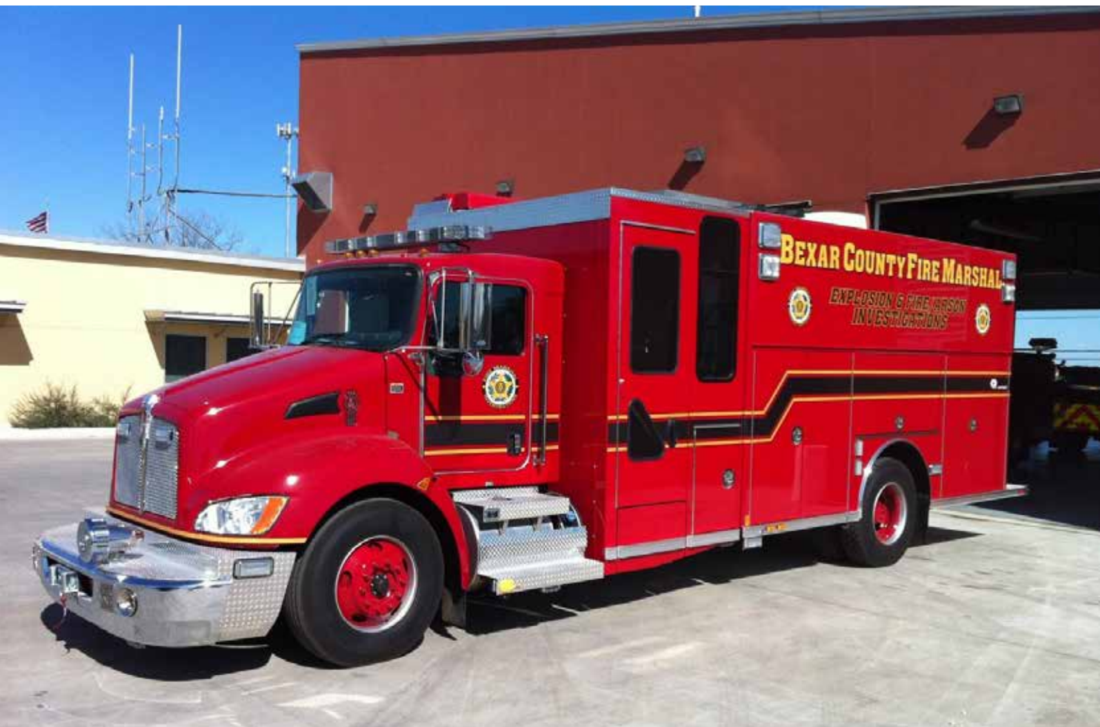
A specialized fire/explosion response vehicle. The truck carries an assortment of tools, evidence collection equipment combined with an onboard interview room. It also doubles as a command post for the investigation of large-scale fire scenes. Photo by: BCFMO
